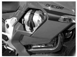
Left: Guzzi's older 1100 motor is bored 3mm and stroked 1.2mm to reach its new '1200' 1151cc size. The pushrod twovalve heads make a bit of clatter until it warms up. but its fuel injection behavior is excellent and no driveline lash is evident at cruising speeds for great drivability. The V-twin sounds great, too.
