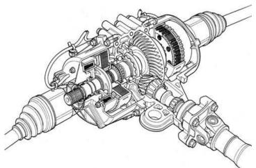
consists of three elements: an electromagnetic coil, a ball-cam device, and a set of 19 wet clutch plates which are similar in design to clutches used in an automatic transmission. Ten of the plates are splined (mechanically connected) to the ring gear while nine of the plates are splined to a half shaft. Left and right clutches are identical.
