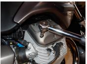
A breather hose is attached to the valve cover. It's located almost invisibly behind the cylinder but is long enough so that you can carefully lift and move the valve cover away without removing the hose. Just be careful, the valve cover gasket is easily damaged at this phase [bad karma warning #3]!
