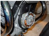
Remove the spark plugs on both sides. Put some paper on the holes to prevent small screws etc dropping into the cylinder
