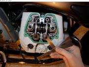
Use thicker and thicker feeler blades until you can feel some resistance while moving the blade between the valve stem and rocker arm. Et voila, this is the valve play on exhaust side. Correct value is between 0.15 and 0.20 mm. You can use the form on the last page to record the measured values.
