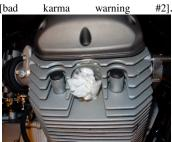
Remove the plastic cover on top of the right cylinder (one allen head screw).
