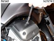
Then unscrew the six valve cover bolts.
